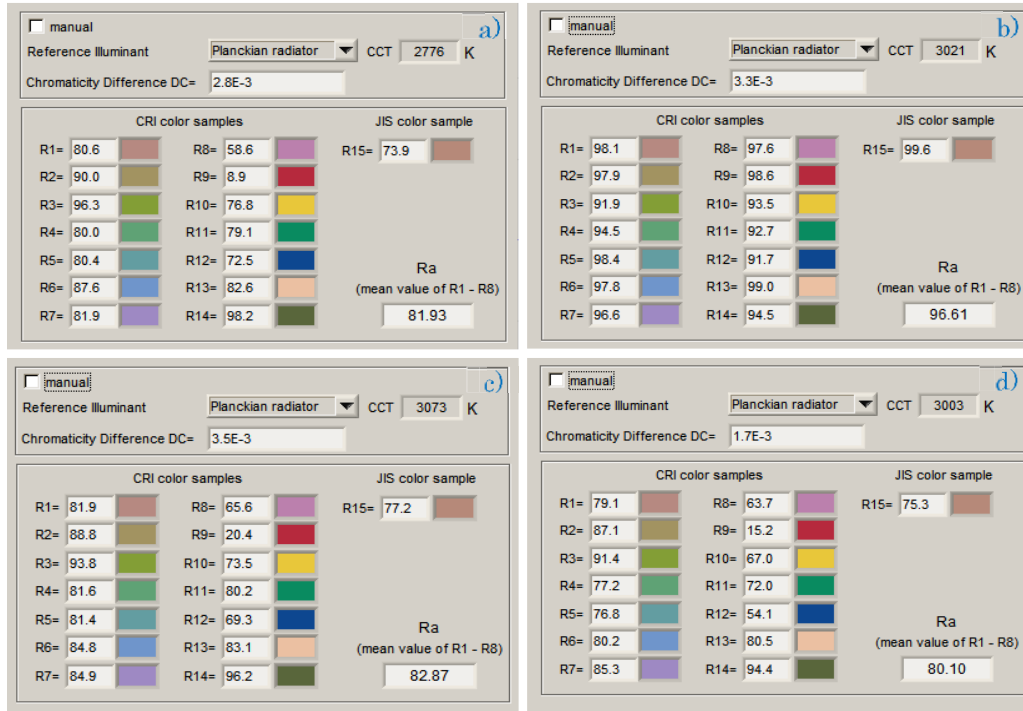
Figure IV.70: Color rendering index a) Cree, b) Osram, c) Philips and d) Seoul.
