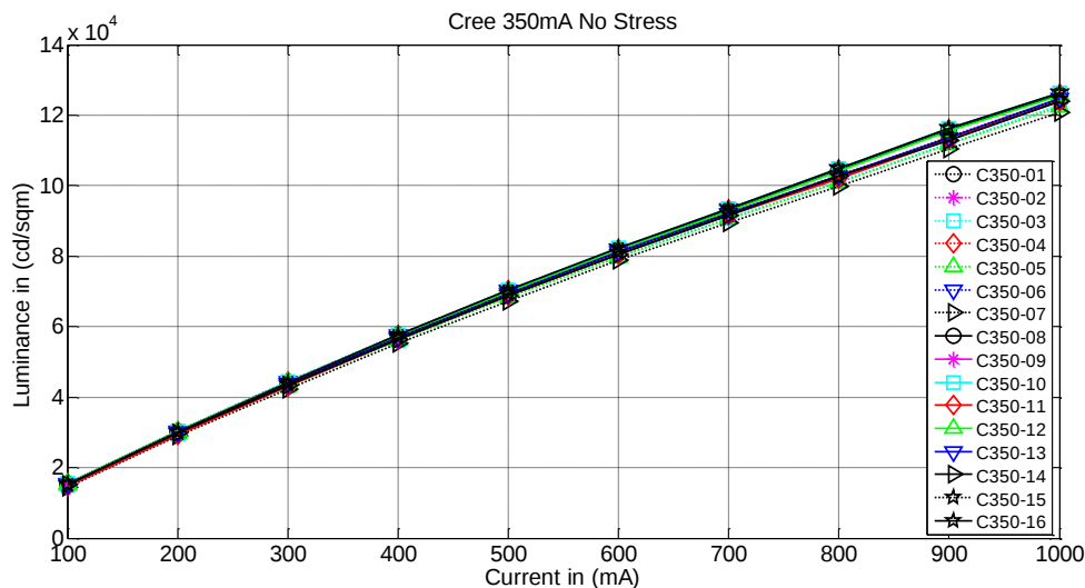
Figure IV.51: L–I characteristic (unstressed Cree@350mA).
