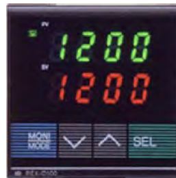
Figure III.8: Temperature controller REX-D100.
