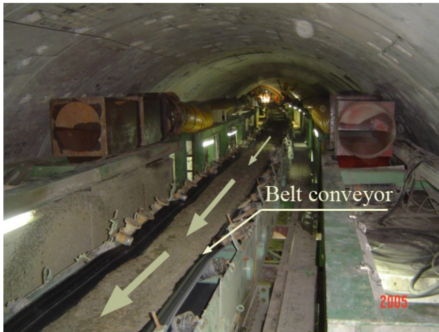
Figure 2.8 Reversing belt conveyor transporting excavated soil (BMA flood diversion project, Saensaep-Latphrao Phrakhanong)
