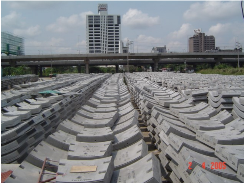
Figure 2.11 Reinforced segmental linings of BMA flood diversion project (Saensaep-Latphrao Phrakhanong)
