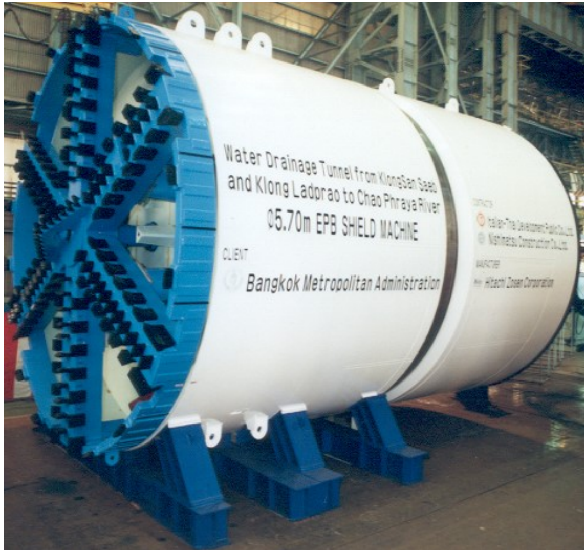
Figure C.1 Articulated EPB shield for MBA flood diversion tunnel (Saensaeplathphrao Phrakhanong project)
