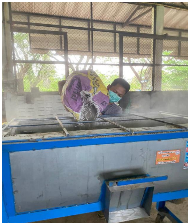
Figure A.7 Concentrate mixing an SM-3.0CR, 3HP, Hz 50, VOLTS 220, AMPS 20.0, r/min 1450, and JIS C 4004 JP 22 JC machine
