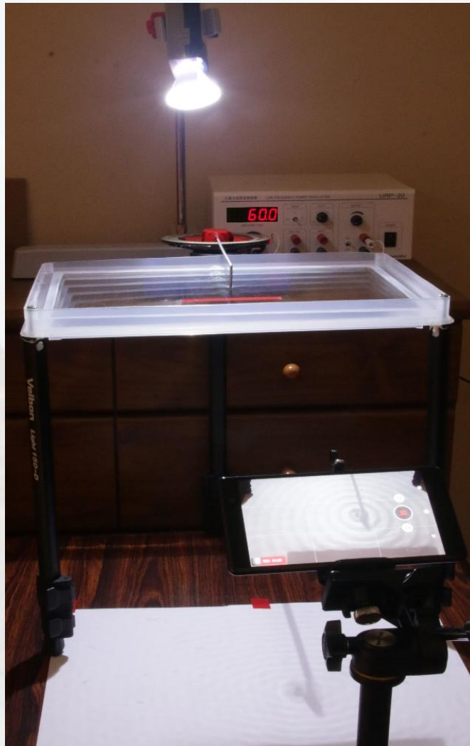
Experimental setup. (a) Tank, (b) LED flashlight and stand, (c) vibrator, (d) signal generator, (e) white paper, (f) coin, and (g) smartphone and tripod.
