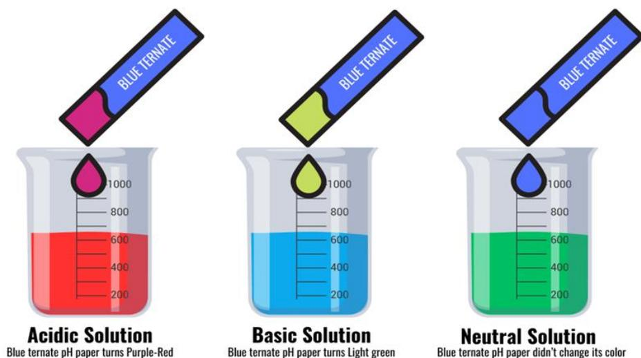
Figure 5 presents the colour responses of natural paper strips infused with Butterfly Pea. The strips turn purple-red in acidic solutions, light green to yellow in basic solutions, and show no colour change in neutral solutions.
