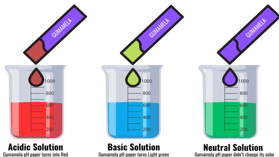
Figure 7 presents the colour responses of natural strips exposed to pH changes caused by household chemicals. The paper strips infused with Gumamela extract showed various colours in different solutions. They turned red in acidic solutions, light green in basic solutions, and showed no colour change in neutral solutions.
